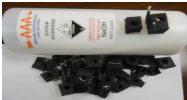
Figure 4: Rubber aggregates conditioned by sodium hydroxide
